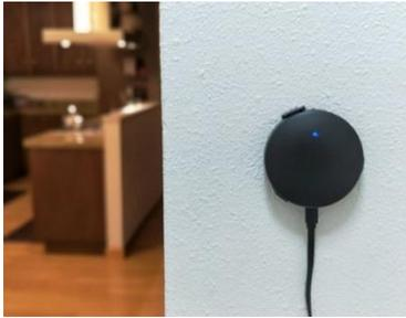
A smart hub is a central control device that connects all smart devices in the home and allows communication among them. For example, homeowners can use a hub to remotely control electric outlets, thermostats, lighting, entertainment, and security through voice activation or smartphone apps. Several applications are also available to allow social connection between family members and
