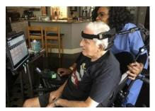
Eye tracking devices are communication and control systems that follow the movement of the eyes and allow individuals with disabilities that restrict speech to navigate through their computer or mobile devices with only eye movements. These assistive technology device applications allow users with physical disabilities to interact with the world with their eyes. Special software allows the person to type by looking at control icons or data displayed on a screen and may include word-
